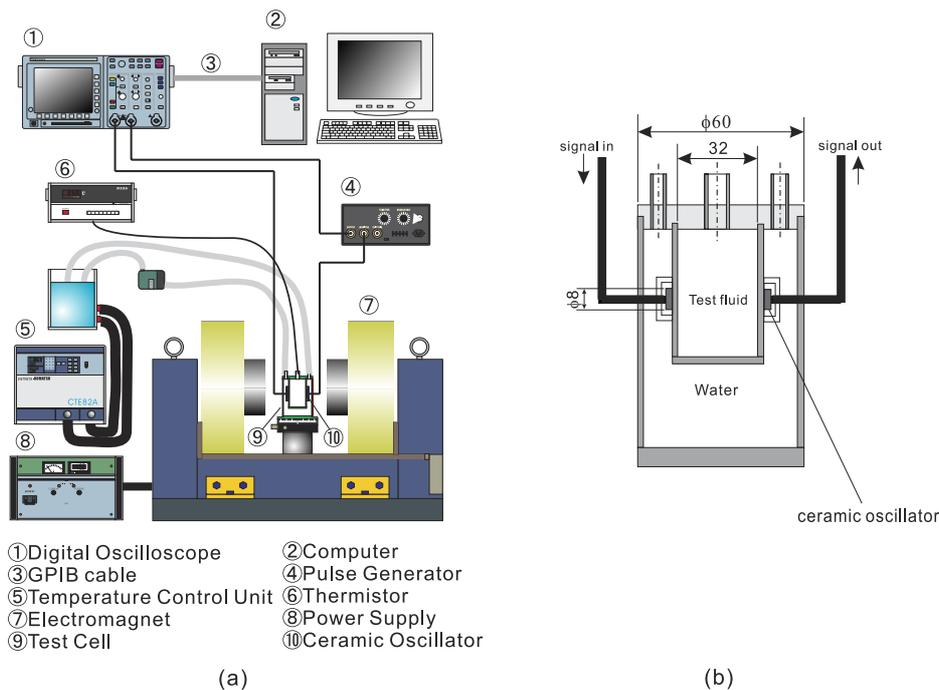
**Figure 1.** Experimental apparatus: (a) block diagram of the apparatus; (b) detail of the test cell in the apparatus.
