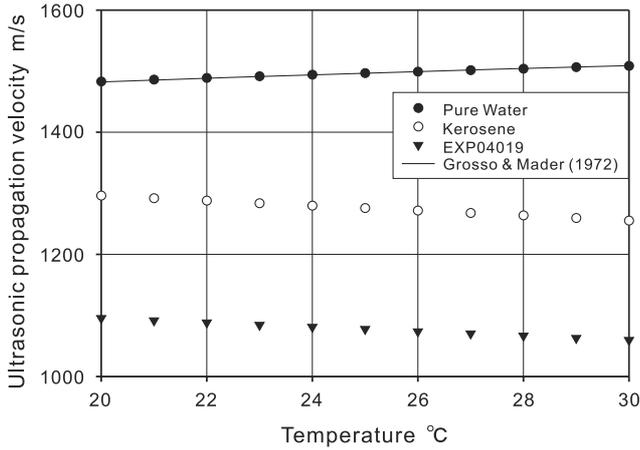
**Figure 2.** Ultrasonic propagation velocity in pure water, kerosene and magnetic fluid.
