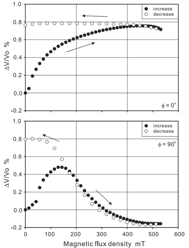
**Figure 5.** Magnetic field dependence of ultrasonic propagation properties—velocity.
